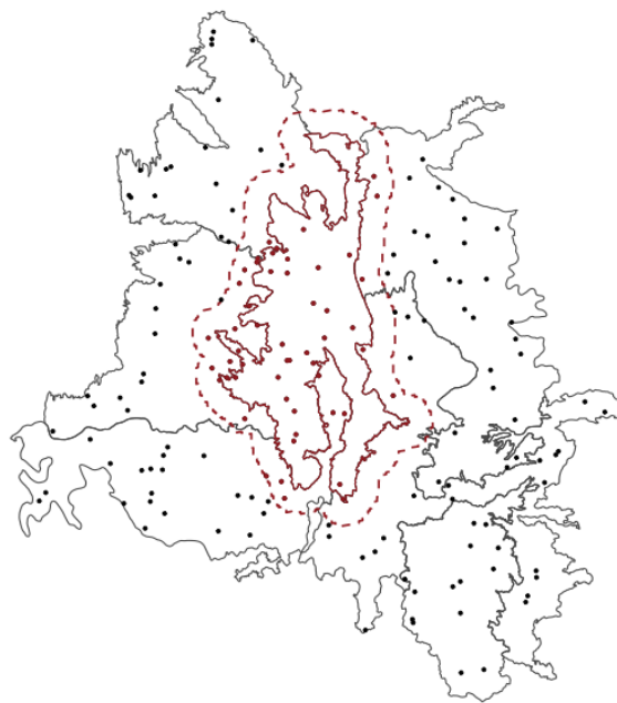
Figure 2: Example showing how observations are selected within a region's buffer zone. Seven arbitrary regions represented as polygons contain 169 observations represented as points. During the regional modeling process, a model is built for each of the seven regions. For this example, all points within 50km of a region are used to build each model. For the highlighted region, all observations within a 50km buffer zone (dashed line) are used to build that region's model. Highlighted points are observations used to build the highlighted region's model.
