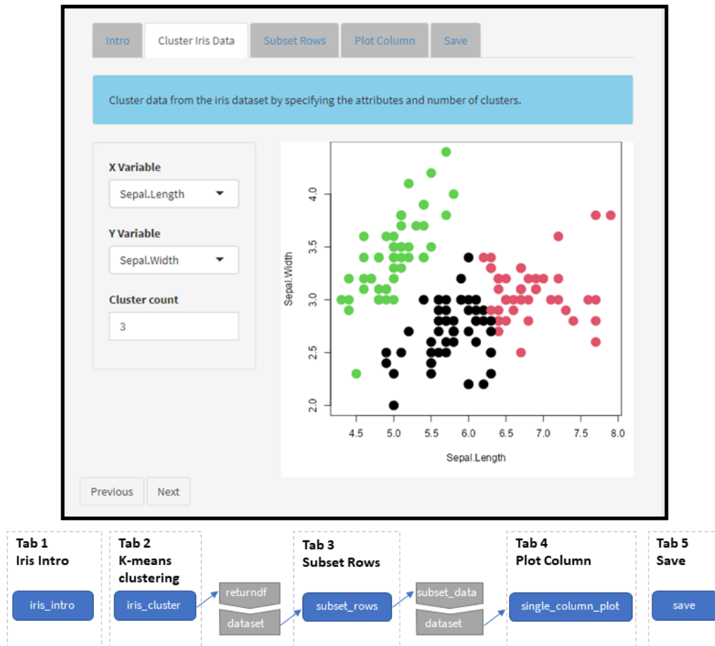
Figure 2: Top: The “iris_explorer” app guides a user through an analysis of the iris dataset in a tab-based sequence. Bottom: A blueprint of the “iris_explorer” app shows the 5 tabs, each containing a single module identified by name within blue ovals. Some of the shiny modules require inputs and generate outputs as identified in gray polygons.
